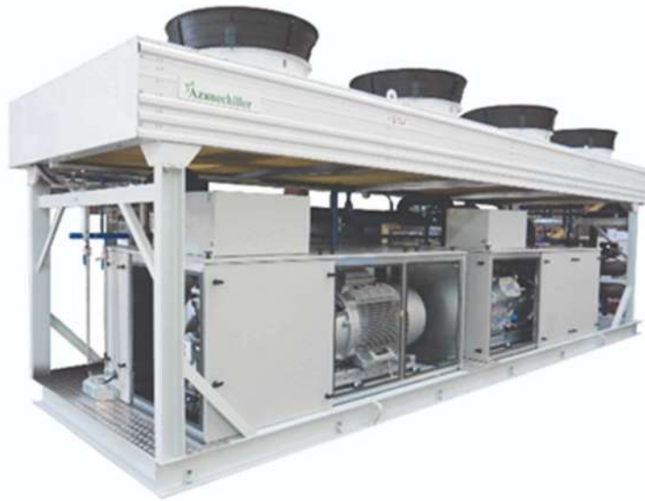
Figure 4. Packaged low-charge ammonia chiller, 40-340 tons (Courtesy: Azane, USA).
