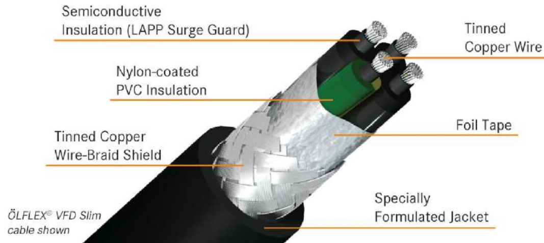
Figure 7. Example of VFD cable. Note the braid, foil shield, ground, and thick insulation on the conductors and jacket. (Image courtesy of Lutze, 2019b.)
