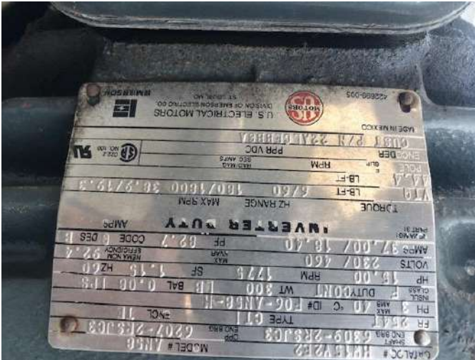
Figure 12. Example of a nameplate on an inverter duty-rated motor.
