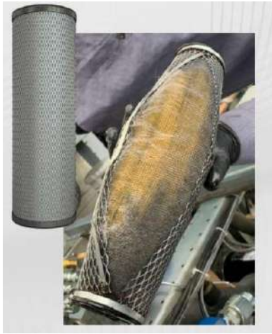
Figure 6. A ruptured filter 5 .
