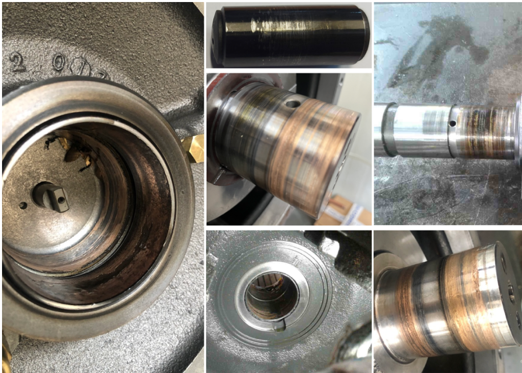
Figure 4. Premature wear on compressor parts caused by wet operation, resulting in insufficient lubrication.
