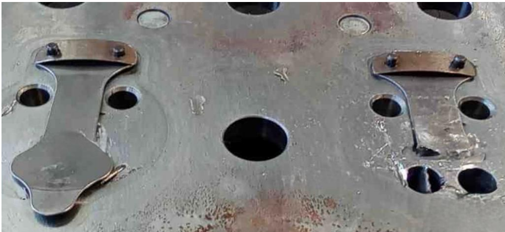
Figure 3. Suction reed after undergoing liquid hammering due to exposure to a liquid slug.
