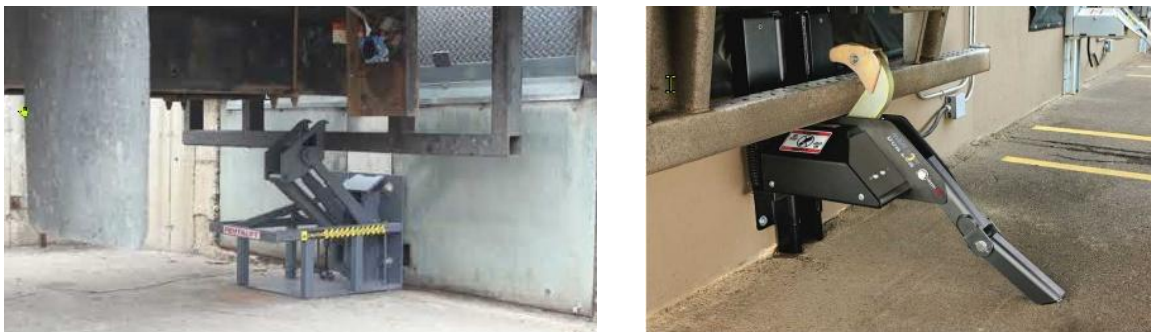
Figure 3. Automatic vehicle restraints with rotating hooks that capture the “RIG”
