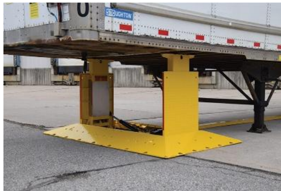
Figure 4. Temporary support (trailer stand)
