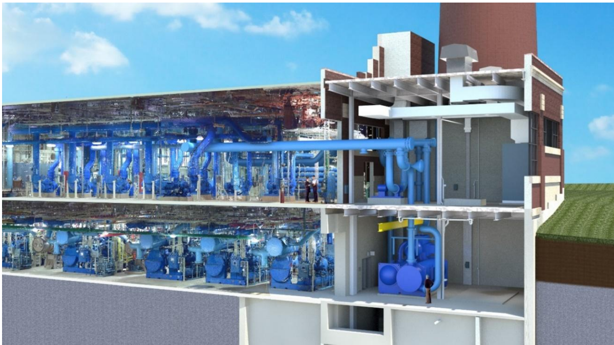
Figure 5: Building cutaway showing a 3D scan integrated with the design model.
